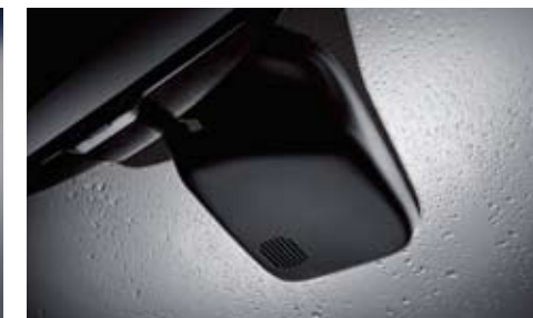
Rain sensor The windshield wipers are automatically activated as soon as moisture is detected for greater convenience and visibility.
